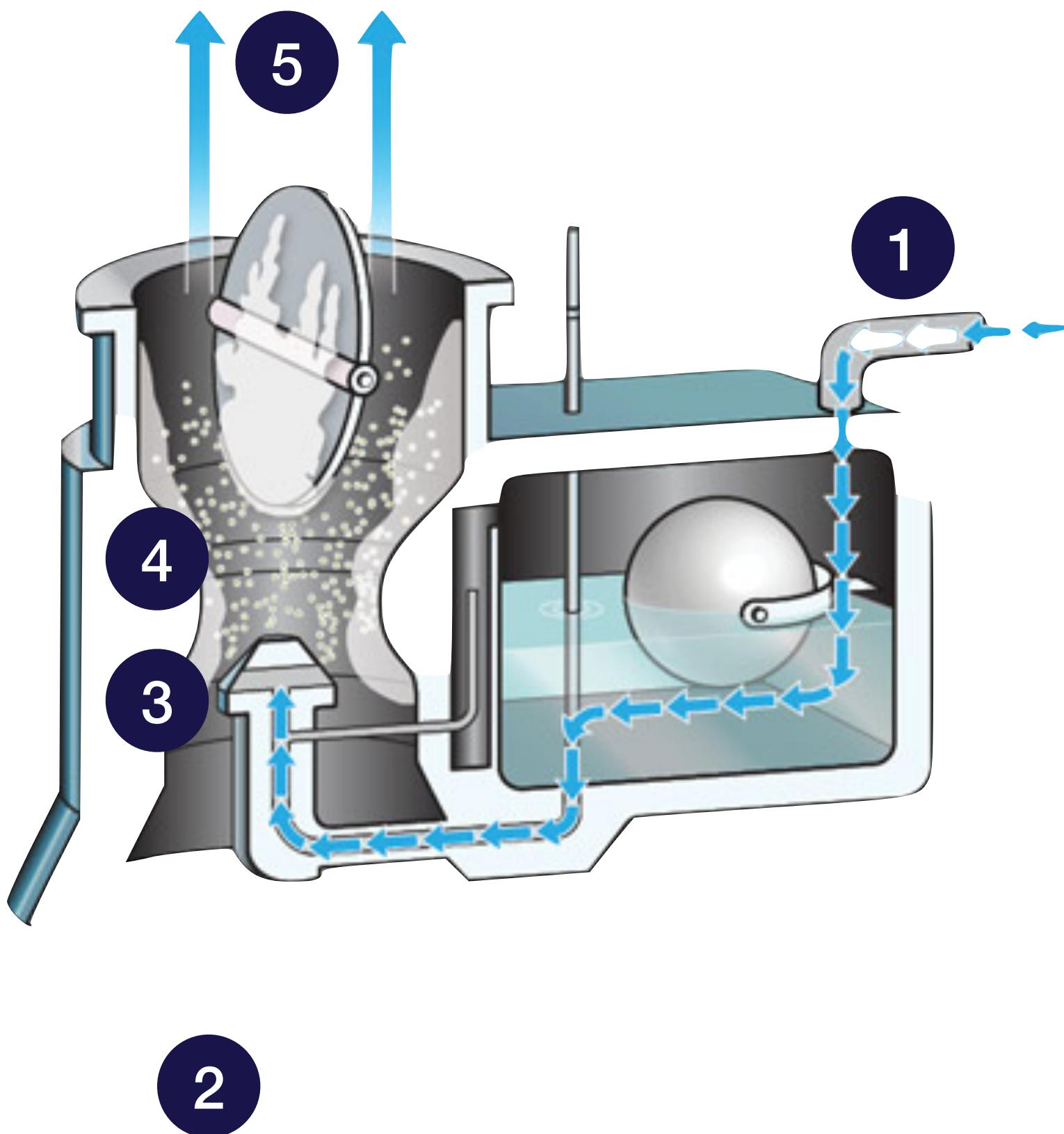
Carburetors are critical components in aircraft engines, particularly in older piston engine aircraft. They play a crucial role in mixing the right amount of air and fuel to create a combustible mixture that powers the engine.
